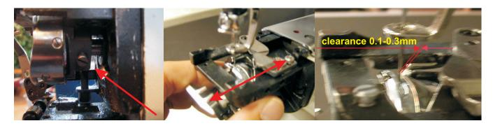
5. Adjust Hook front to back (clearance between Needle to Hook tip 0.1mm to 0.3mm) Also adjust Hook right to left (needle must be on the center of the Hook tip)
