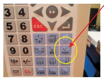
Select 100<sup>0</sup> Degree to reset the needle position again
