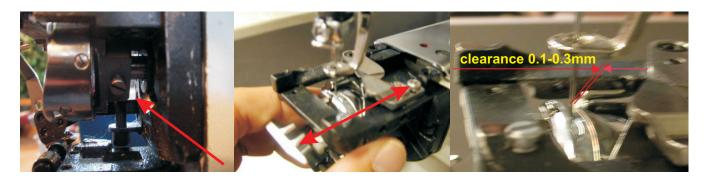
5. Adjust Hook front to back (clearance between Needle to Hook tip 0.1mm to 0.3mm) Also adjust Hook right to left (Hook tip must be behind the center of the Needle)
