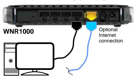
Avoid using NETGEAR instructions to install the router. Just plug the router into the LAN port on your computer. Go to the Network connections in your computer and open the Local Area Connection (Not the Wireless connection if it exists. You may need to Disable the wireless connection). Right-click the connection and choose Properties. Select Internet Protocol TCP/IP and click Properties.
