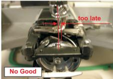
6, Then tighten 3 screw firmly use serten size of screw driver
